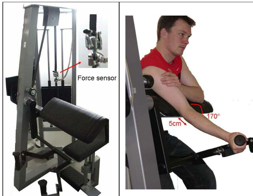
Figure 2. Test machine with force sensor (left); Right: measurement position.
