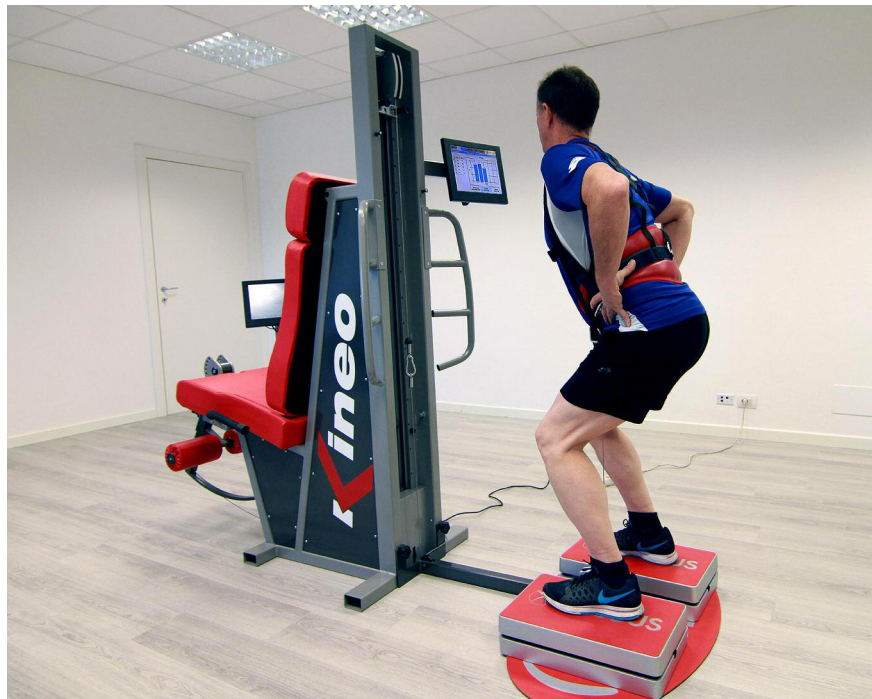
Figure 1. During the IYYT the subject is bound to the equipment via the yo-yo cable which offers a supramaximal resistance making isometric the push movement. Two synchronized force platforms (Thesis System, Globus Italy. Reliability of the measure: 0.5 Kg; error of device: <1%; sample rate 1000 Hz; sample depth 140 bit) record the isometric strength value during the push performed by the subject.
