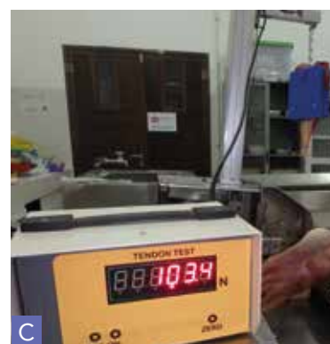
Figure 4. Achilles tendon secured onto a tensile testing machine (A, B). The monitor showed the ultimate strength (C).
