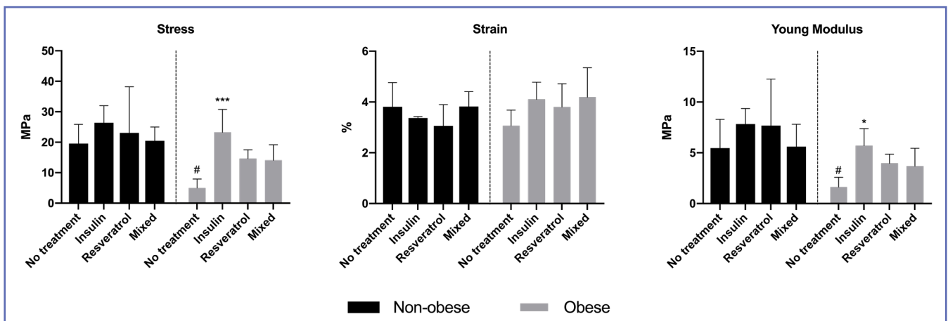
Figure 4. Stress and Strain values of the evaluated tendons. No significant difference could be observed in the strain of the different groups. Obesity alone decreased the tendon strength when compared to all non-obese animals (#). Insulin treatment made the tendon as resistant as the non-obese animals' tendons.
