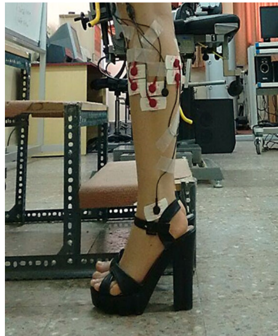
Figure 1. Electrode placement with high heeled shoe. Tibialis Anterior (TA): four finger-breadths below the tibial tuberosity and one finger-breadth lateral to the tibial crest, Peroneus longus (PL): three finger-breadths below the fibular head directed toward the lateral aspect of the fibula. Gastrocnemius medialis (GM): as far as a palm below the popliteal fold on the medial side of the calf muscle.
