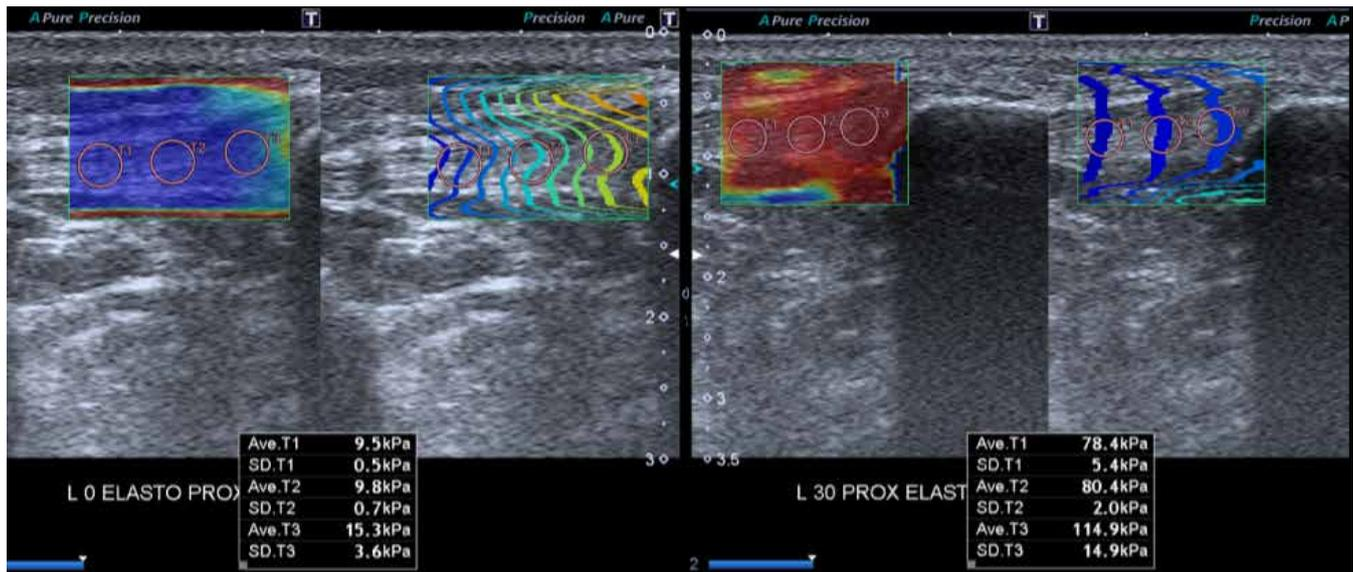
**Figure 2.** Shear-wave elastography images from the proximal part of the patellar tendon. (A) 0 degrees, (B) 30 degrees of knee flexion.
