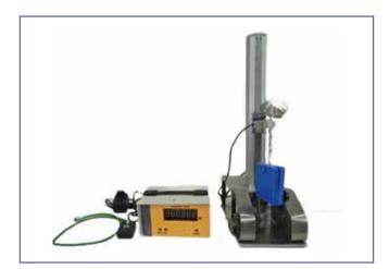
Figure 3. Tensile testing machine
