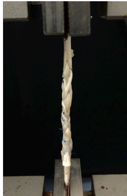
Figure 5. All sutured tendons were subjected to cyclic loading test using a tensile testing machine (AG-Xplus; SHIMADZU Corporation, Japan).
